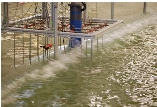
1450 Figure 10: Breaking wave impact at a monopile from model tests of the DeRisk project (Source: Bredmose et al., 2016)
