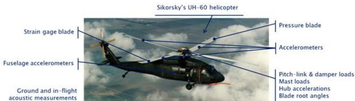
Figure 7: A highly instrumented UH-60A flying over the San Joaquin Valley in California during the UH-60A Airloads Flight Test Program. The data set collected in these experiments led to major advances in the modeling and simulation of rotorcraft vehicles. Wind energy science needs similar high-quality, fully open-access data sets, which are indispensable for validating the models and tools that will enable the design of the wind turbines of the future. (Photo from https://rotorcraft.arc.nasa.gov/Research/Programs/uh_60_program.html )
