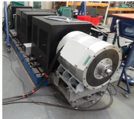
Pseudo-magnetic direct drives (5, 16 and 200 kNm demonstrators)
