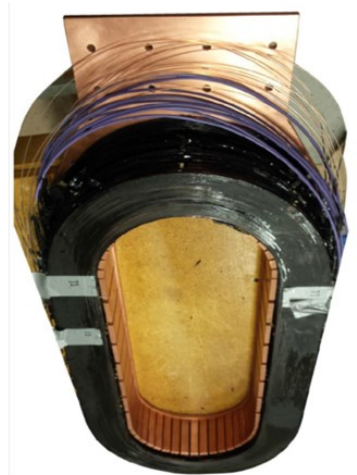
High-temperature Superconducting generators, MgB 2 race track coil & 20MW concept
